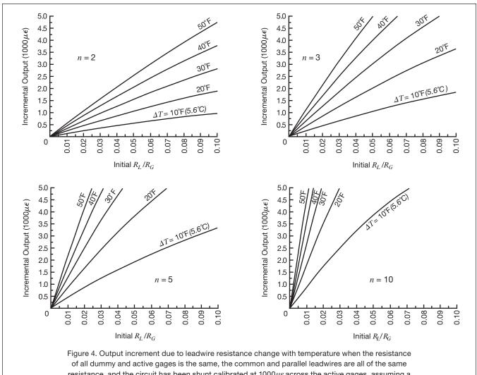
resistance, and the circuit has been shunt calibrated at  $1000\mu\varepsilon$  across the active gages, assuming a gage factor (package data) of 2.000. Note that any thermal output from the strain gages is not included.
