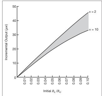
Figure 3. Range of nominal incremental output produced in companion parallel circuits by a strain change of  $1000\,\mu\varepsilon$  in any one circuit when the initial resistance of all active and dummy gages is the same, common and individual leadwires are all of the same resistance, and the circuit has been shunt calibrated at  $1000\,\mu\varepsilon$  across the active gages, assuming a package gage factor of 2.000.
