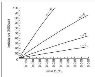
Figure 2. Initial imbalance produced by the use of a common leadwire when all active and dummy gages are of the same resistance, common and individual leadwires are of the same resistance, and the instrument gage factor setting is 2.000.
